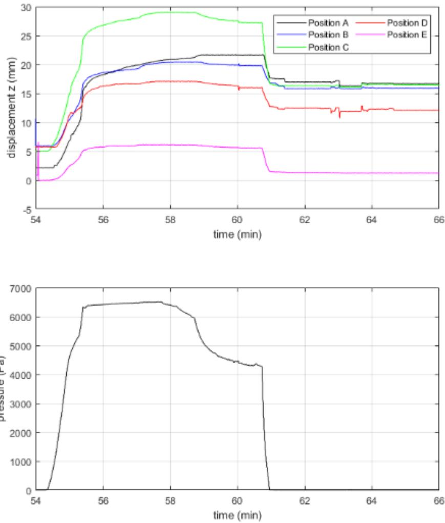
Figure 3: Displacement and pressure for the second test from 0 Pa to 6500 Pa.
