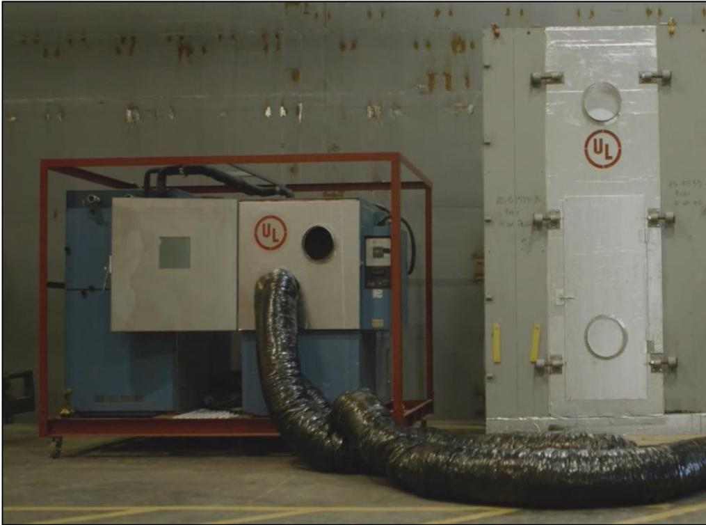
**C-03 Test bench for extreme thermal conditioning and freeze/thaw**
