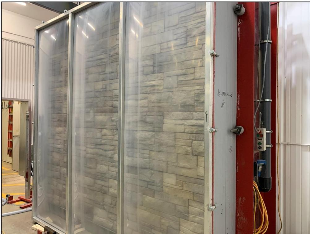
**C-02 Taking leak measurements from the test bench during airtightness tests**
