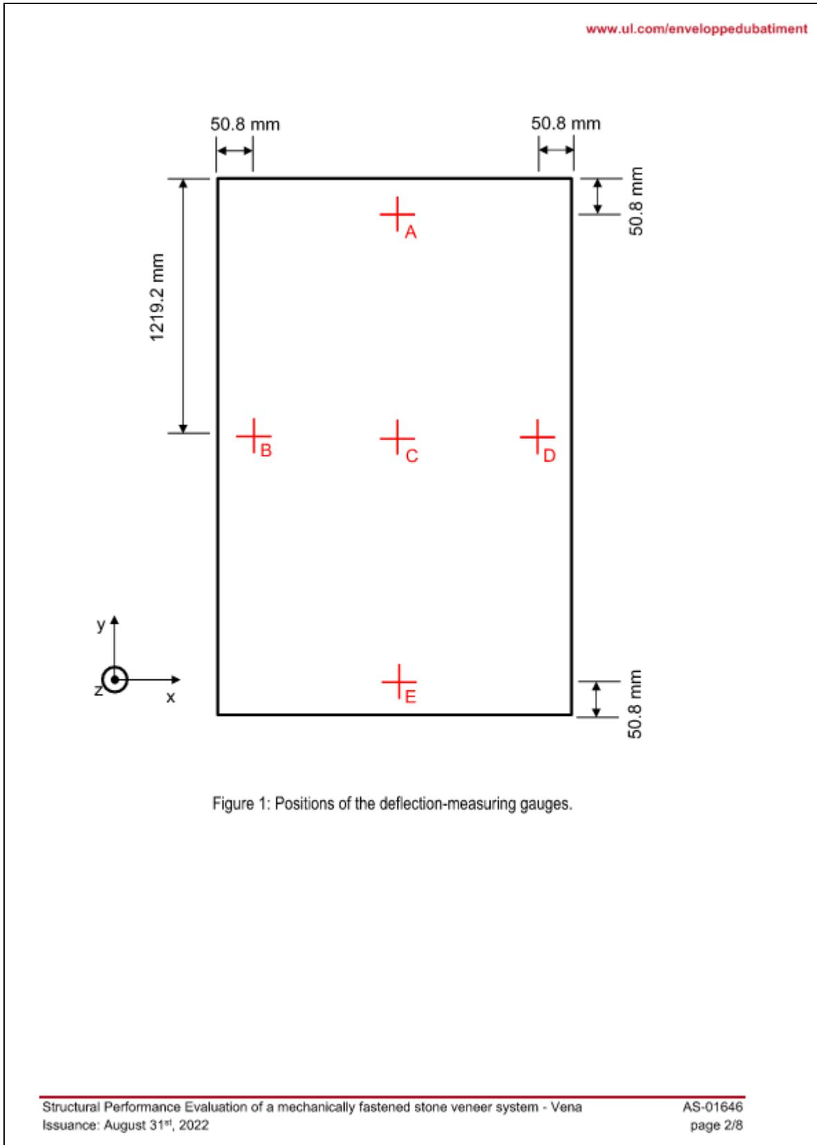
Figure 1: Positions of the deflection-measuring gauges.
