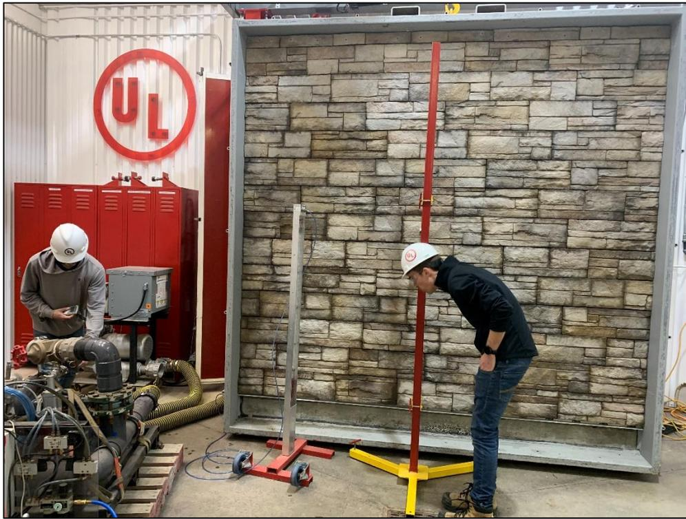
**C-07 Wind Load Cyclic Pressure Test**
